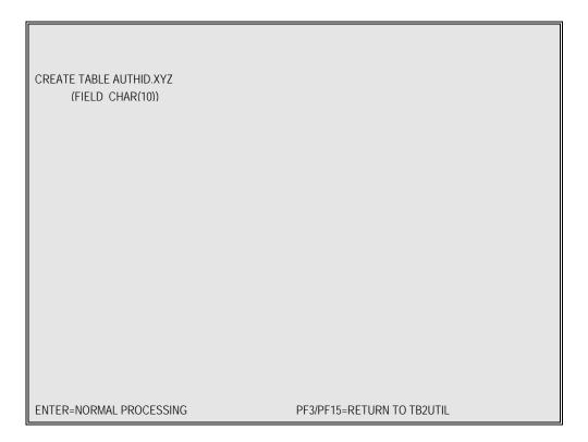
STEP 16. A successful SQL processing message as shown below will appear or an SQL error message preceded by a negative number will be returned. Either of these two events signify a completed DB2 action and verify that TABLES/AS is functioning correctly.
