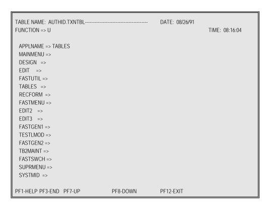
STEP 7. Change function code to C and transaction names that are to be changed and press ENTER.
